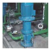
Discharge and transferpumps for PUR raw materials.
